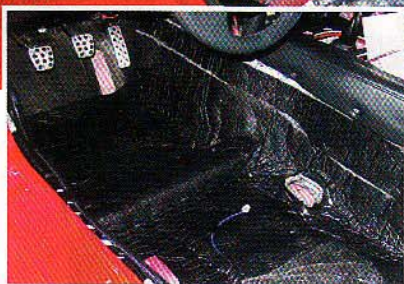
SOUND OFF: With Brown Bread now covering as much of the S2000 as possible, the carpet and underpad can now be put back in place.
